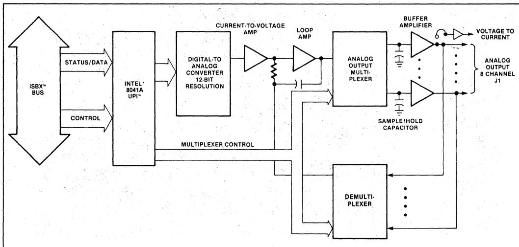
Figure 1. iSBX 328 Analog Output MULTIMODULE Board Block Diagram
